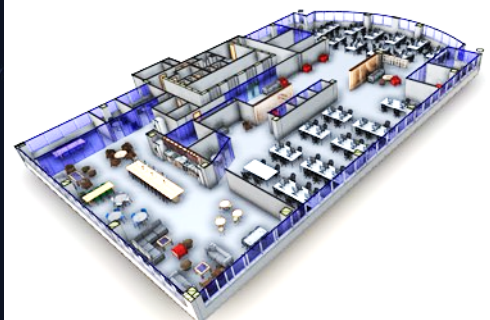
Scan to BIM for office project: Point cloud (left) captured by one person in 40 minutes. 3D BIM model created in Revit.
